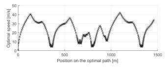
Fig. 7. Racing line optimal speed profile without constraints on the maximum speed.
