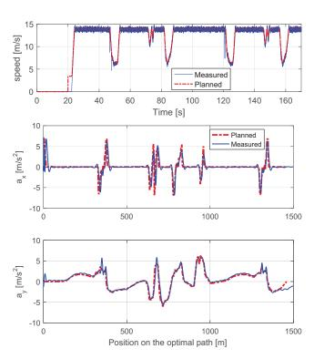
Fig. 10. From the top: speed tracking over two laps, detail of longitudinal and lateral acceleration tracking.
