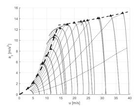
Fig. 6. Map of Achievable Performance [24] for the lateral acceleration. Continuous grey lines represent data from slow ramp steer maneuvers performed on the vehicle dynamic simulator. Thin dashed lines represent points at the same value of steering angle, increasing from the bottom to the top. The thick dashed line fits the peaks of the steer maneuver data and gives a conservative limit on the lateral acceleration as a function of the longitudinal speed.
