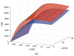
Fig. 4. Axle characteristics obtained with the Pacejka Tyre Formula [26]. (a) A detail of the model fitting data from a real track compared with the data from the car simulator. (b) front (blue) and rear (red) axle characteristics as a function of longitudinal speed and apparent slip angle.
