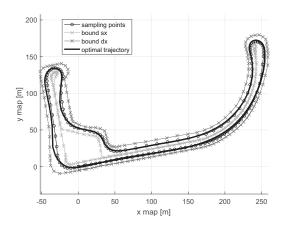
Fig. 5. Racing line in map frame  $p_{map}^*$ , with approaching path from zero speed at (x,y)=(0,0).
