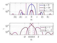
Fig. 7. Zero-dynamics equilibria for intermediate values of  $\gamma$  and various desired tip orientations  $\bar{q}_0$ . Equilibria are found intersecting  $\xi = \Gamma_2(\bar{q}_0, q_1)/(6\bar{q}_0 - 12q_1)$  and  $\xi = \gamma$ . The upper plot reports the graphs for  $\bar{q}_0 \in \{-2\pi, 0, 2\pi\}$  and the lower one for  $\bar{q}_0 = \{1, -1\}$ .
