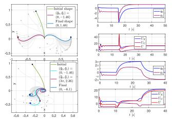
Energy-injection-based control of SIP with  $\gamma = 0.05$  (top) Fig. 11. and  $\gamma = 0.005$  (bottom). Left-side graphs show the SIP trace in the Cartesian coordinates as the SIP moves with time, top-right plots the temporal evolution of  $q_0$  and  $q_1$ , and bottom-right those of the potential energy terms  $(U_K, U_G, \text{ and } U)$ .
