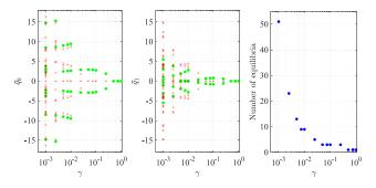
Pattern, stability, and number of equilibria with no external Fig. 2. input ( $\bar{\tau} = 0$ ). From left to right, the first and second plots illustrate the location and stability of the equilibrium pairs  $(\bar{q}_0, \bar{q}_1)$  against the bifurcation parameter  $\gamma = k/mgL$  (stable equilibria are painted in green and unstable ones are marked in red); the third plot reports the trend of the equilibrium number.
