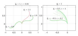
Fig. 9. Cartesian (*x*, *y*) shapes of the SIP with intermediate tip orientation ( $\bar{q}_0 = 1$ ). The left plot displays the three possible zero-dynamics equilibria for  $\gamma = 0.05$ , while the right plot is intended to show how the unique equilibrium varies for values of  $\gamma \ge 0.1$ . Stable equilibria are in green and the unstable one is in red.
