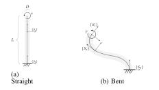
Fig. 1. This letter analyzes the structural properties of the soft pendulum with affine curvature, with a special focus on collocated control. This template model has two degrees of freedom and one degree of actuation, and it presents a soft version of the rigid acrobot.
