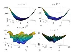
Fig. 5. Potential energy forms for various values of the bifurcation parameter  $\gamma$ . The figure highlights the radially unbounded behavior of *U*; analytically speaking, while  $U_G$  is bounded via the Lagrangian description of the SIP [4],  $U_K = \frac{1}{2}q^T Kq \rightarrow \infty$  for  $||q|| \rightarrow \infty$ .
