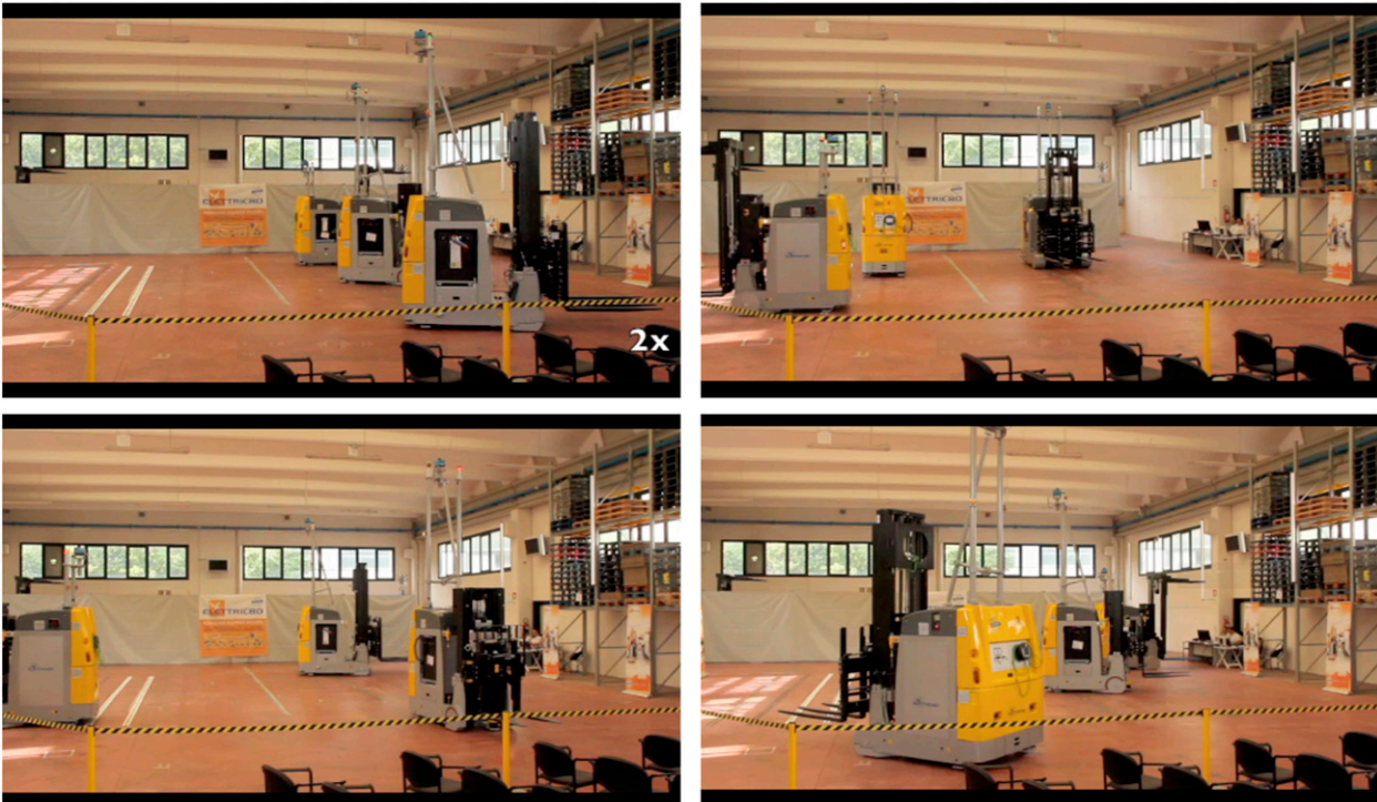
Figure 4. Warehouse case-study. Highlights from the experiment with three commercial LGV within a representative industrial plant. The onboard low-level control of each LGV is encapsulated via software as a black box to represent the decoder map of the system; the supervisory control system is programmed in C# for high-level control of the vehicle to implement the functions of the encoder map s_i , detector map e_i and automaton map \delta_i . Once the source code of these three components is written, the local monitor and consensus nodes are generated via the tool described in Appendix D and then linked with the object code of the decoder map to the Beckhoff TwinCAT3 target machine. Experiments have been performed at the premises of the Italian company Elettric80 SpA.
